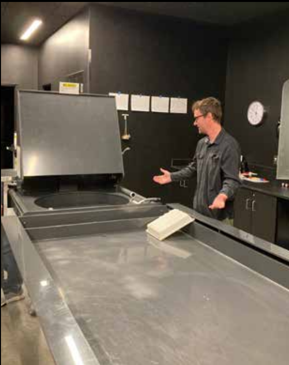
A long "sink" in the middle of the room that Shawn Bush , photography instructor, explained, this is where the developing chemicals are mixed and placed in the trough to develop the actual photographs. The chemicals are quite toxic, and this trough is the most advanced one available. Note the "slots" near the top along each side of the trough. These slots suck out the toxic vapors created by the chemicals, thereby protecting the students. The size of the table allows many students to develop photographs at the same time.
