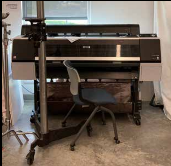
Above is the state-of-the-art 44-inch printer that is able to print a photograph 44 inches wide and as long as one wants since the photo paper is on a roll.
