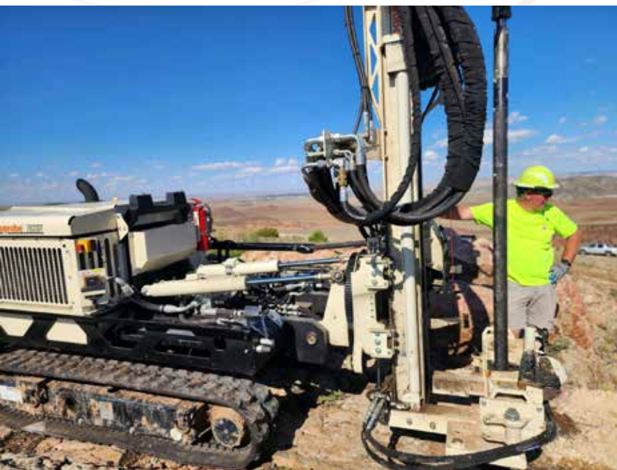
Bradley Carr, associate research scientist, University of Wyoming, Department of Geology and Geophysics, is shown with the drilling unit brought in by the University of Wyoming to dig several core samples from some of the meteorite locations. (Courtesy photo/Kent Sundell)
